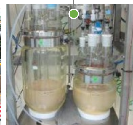
Small Volume Continuous (SVC) Manufacturing in Fumehood at Kinsale
